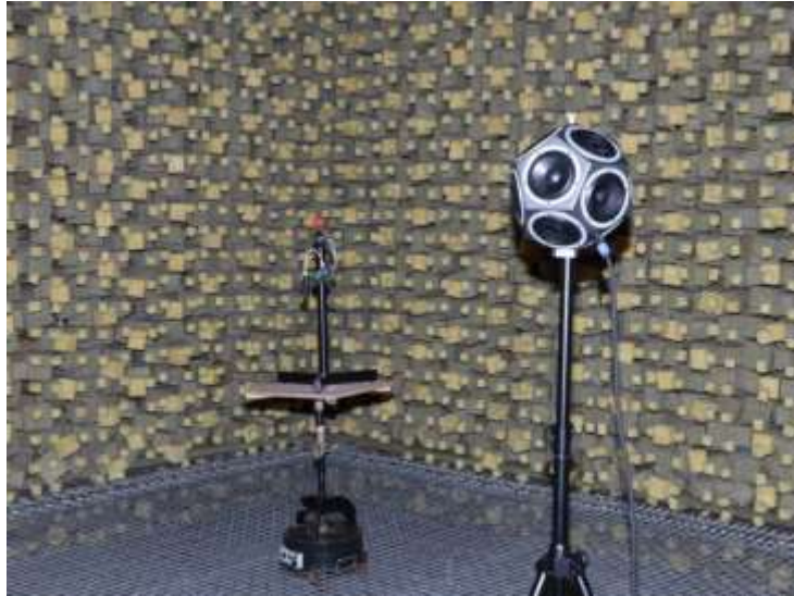
Figure 15. Sound source applied in measurement in anechoic chamber
