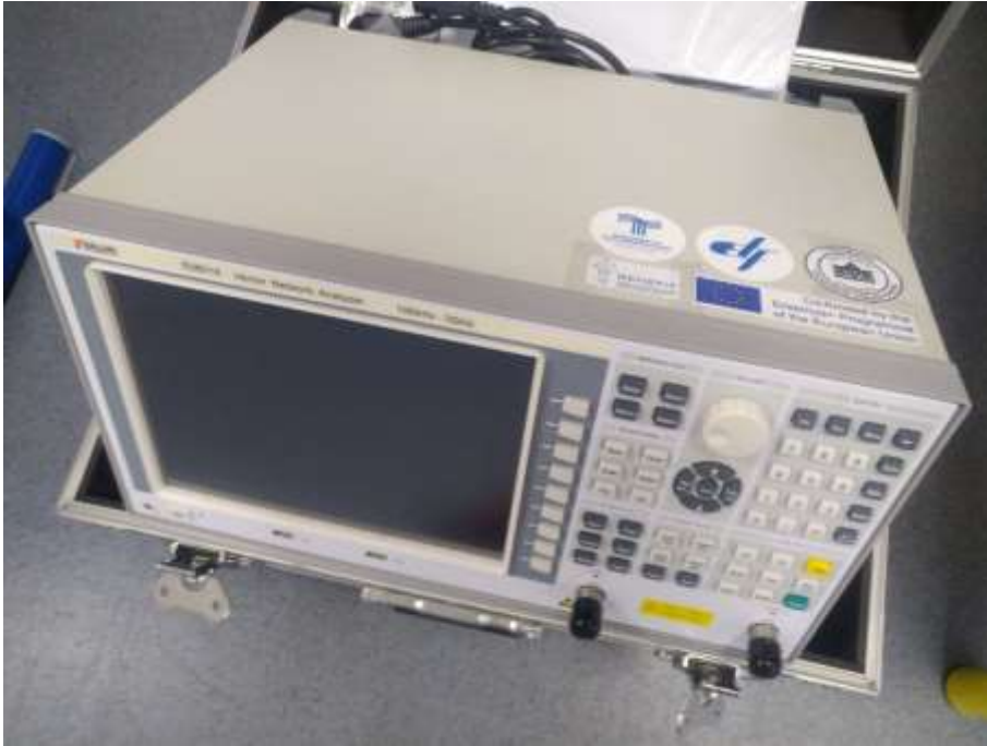
Fig. 6 Vector Network Analyzer 100kHz - 3.2GHz with the Calibration kit
