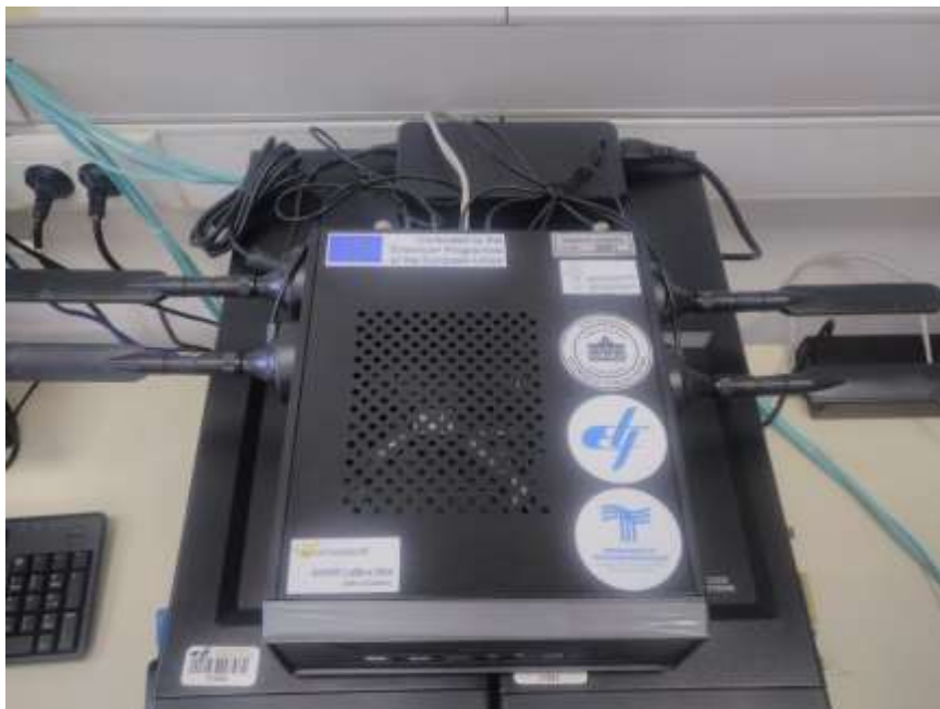
Fig. 5 Software-based LTE base station running on a computing machine for the telecommunication lab: Amari LTE 100 eNodeB + EPC Software 4G network
