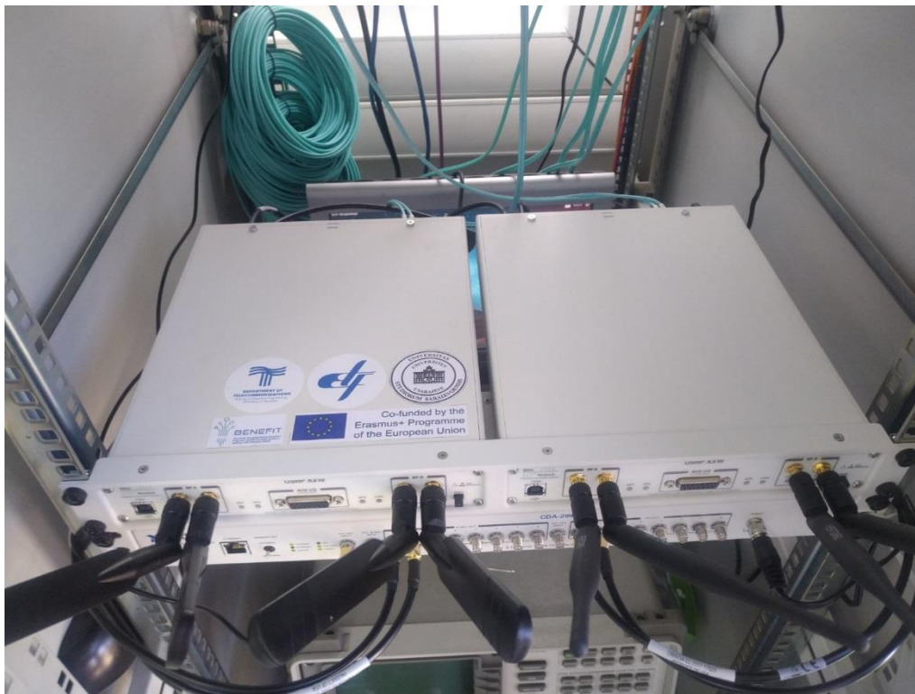
Fig. 7 High-performance software defined radio equipment: USRP X310 and USRP N210
