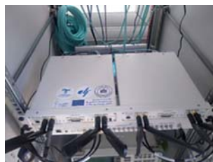
Figure 4.2. Software-based LTE base station, Vector Network Analyzer 100 kHz, SDR equipment (UNSA)
